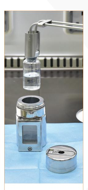
This **light weight** (less than 1 kg) and **compact-sized** Cont'Elu pot can also be used as a conventional vial shield for various daily radiopharmaceutical preparations.
