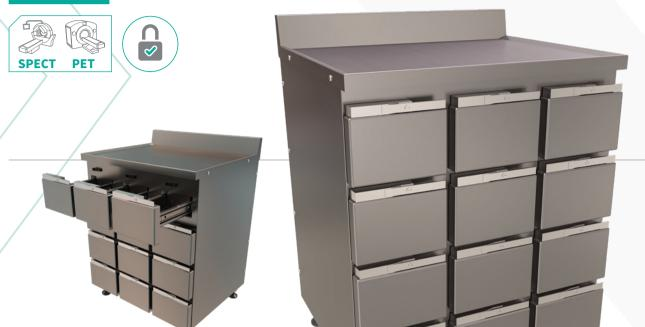
The storage unit is dedicated to the secure containment of radioactive sources for services handling many different radioactive isotopes. It consists of nine independent shielded sliding lockable drawers. It is more functional than a standard storage system, thanks to its size and large storage capacity, and also offers a large, flat preparation area, for improved user comfort on a daily basis.
